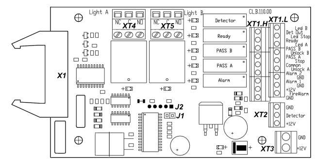
Figure 5. Control Logic Board (CLB)
