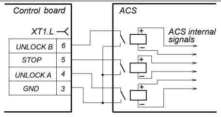
Figure 6. ACS control element — normally open relay contact
