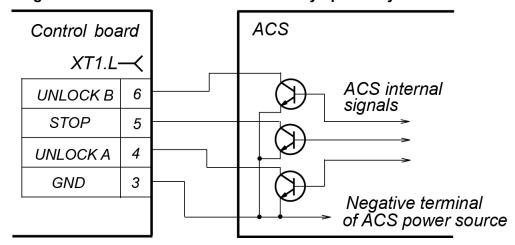
Figure 7. ACS control element — circuit with open-collector output
