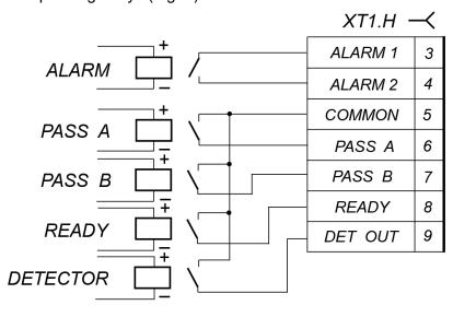
Figure 8. Output cascades for PASS A, PASS B, Ready, Det Out and Alarm
